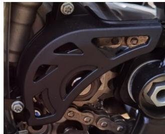
The image above is an example of an OEM front sprocket guard. After-market guards are acceptable so long as they provide similar protection.
